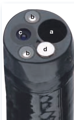
Figure 2 Distal tip of video endoscope; note the working channel (a), fibreoptic light guide (b), lens (c) and air/water nozzle (d). ©2013 Courtesy of KARL STORZ GmbH & Co KG
