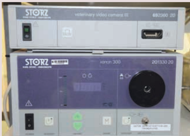
Figure 10 A single camera control unit (top) and xenon light source (bottom) with connector for a fiberoptic light cable
