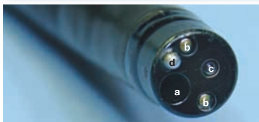
Figure 6 Tip of video endoscope insertion tube. (a) Working channel, (b) light source, (c) viewing lens/CCD chip and (d) air/water channel
