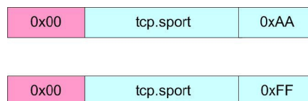
Figure 4. The two special packets (ISN_EMPTY and ISN_NEW_BLOCK).
