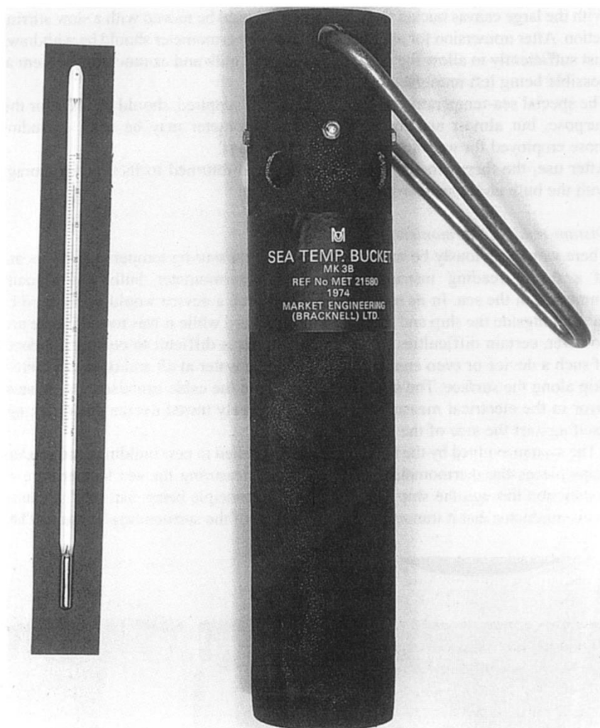
Figure 15. Sea temperature bucket and thermometer.
