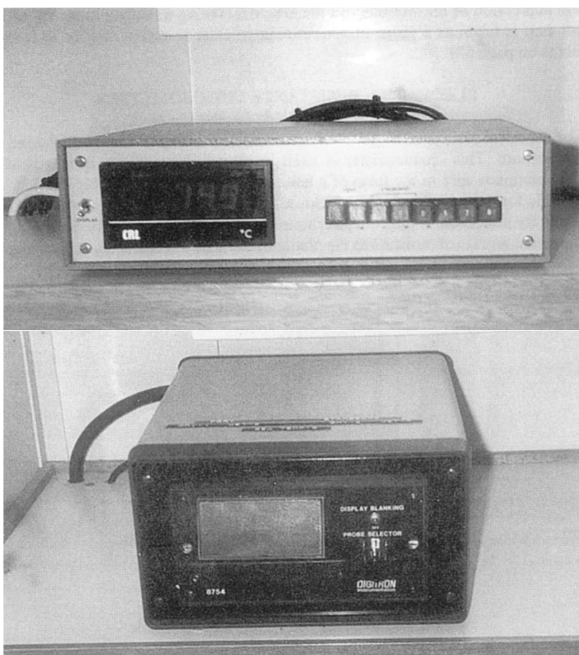
Figure 13. Digital Temperature Indicators. Top Mk.1B, bottom Mk.2
