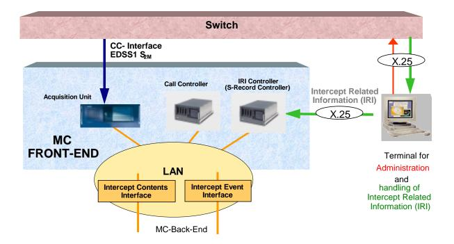
Figure 4-2: Example of Front-End for active monitoring
