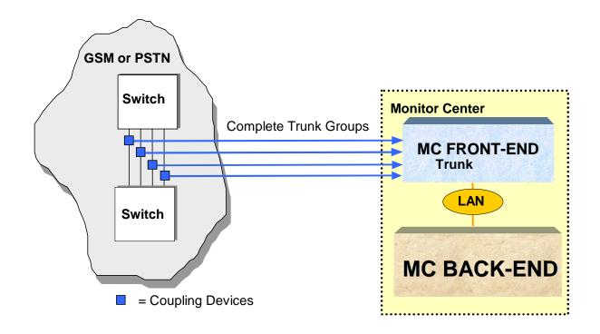
Figure 2-2: Passive Monitoring: Connection MC into the Communication Network
