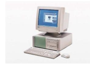
The Supervisor Station is a WIN NT based Desktop PC and can be used to mark subscriber in a passive monitoring scenario. The Supervisor can only be used by CAS signalling, SS#7 is not supported. The use of a supervisor is advisable if beside trunk monitoring also a Siemens EWSD active monitoring Frontend is necessary because the Supervisor is also capable to do the monitoring administration (marking of subscribers) of one or more EWSD switches (see 5.2.2.1).
