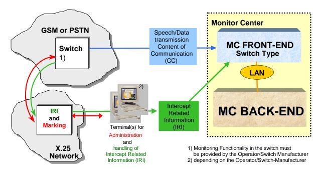
Figure 2-1: Active Monitoring: Connection MC into the Communication Network
