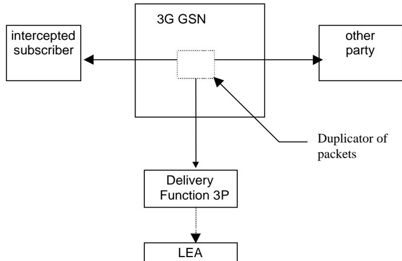
**Figure 20: Configuration for interception of Packet Data product data**
