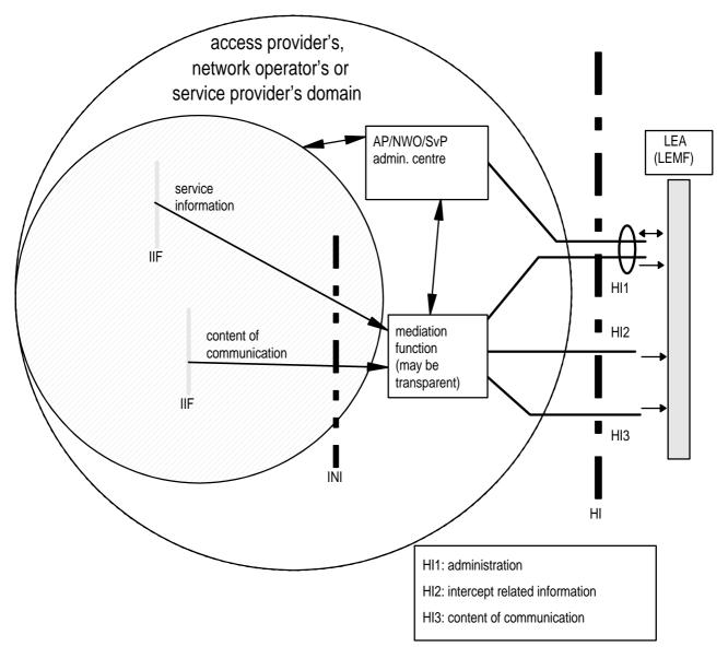
Figure 3: NWO/SvP functional block diagram showing HI
